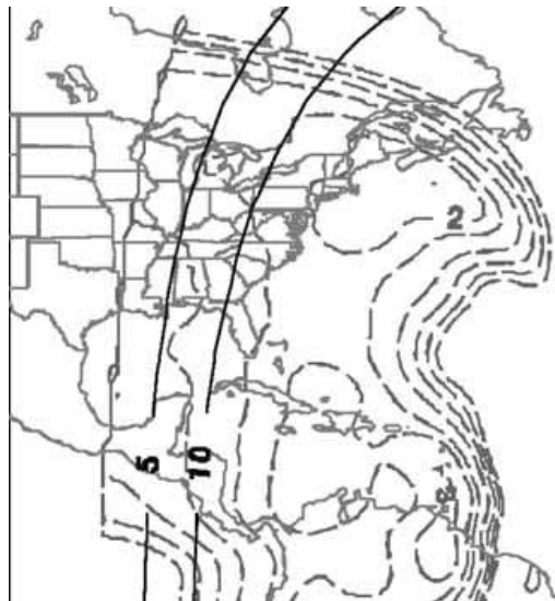
Figure 5 Uplink gain for Telstar-12 (source: Loral Skynet Telstar 12 Technical Manual). The satellite has the same sensitivity to transmissions from much of Cuba, the apparent source of the most recent jamming, as the authorized uplink site near Washington D.C.
