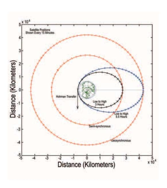
Fig. 2: Maximum Altitudes and Time-to-Apogee for North Korean Direct Ascent Anti-Satellite Attacks with Scud-C and **Nodong Ballistic Missiles**
