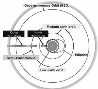
Highly idealized depiction of natural radiation belts. Inclination of each satellite orbit set to zero for display purposes.
